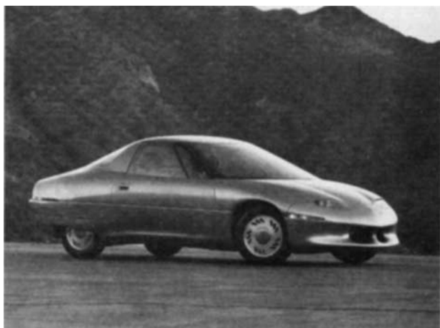
Fig. 3. The General Motors "Impact" prototype electric vehicle. Environmental issues and a declining availability of petroleum are forcing serious consideration of electric and hybrid automobiles. These vehicles will require new materials and technologies for electrical storage and use, for lightweight, aerodynamic construction, and for safe operation.
