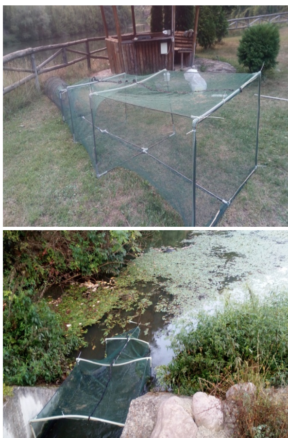
Fig. 2. Fish trap for studying the upstream fish migrations through the fish passes. Upper – general view; Lower – working position.
