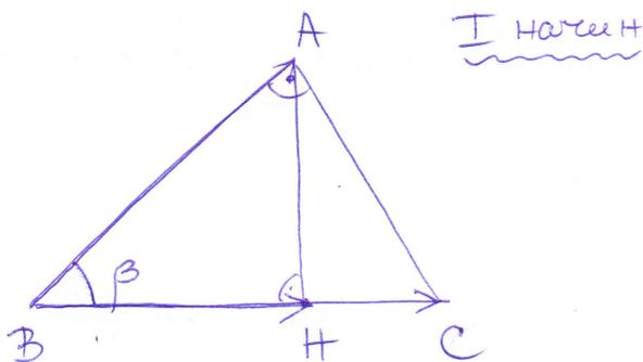
$$\begin{aligned} \|\vec{BH}\| &= \text{proj}_{\vec{BC}} \vec{BA} = \\ &= \frac{\vec{BA} \cdot \vec{BC}}{\|\vec{BC}\|} = \frac{100}{5\sqrt{5}} = \frac{20}{\sqrt{5}} \\ &= \frac{20\sqrt{5}}{5} = 4\sqrt{5} \end{aligned}$$
