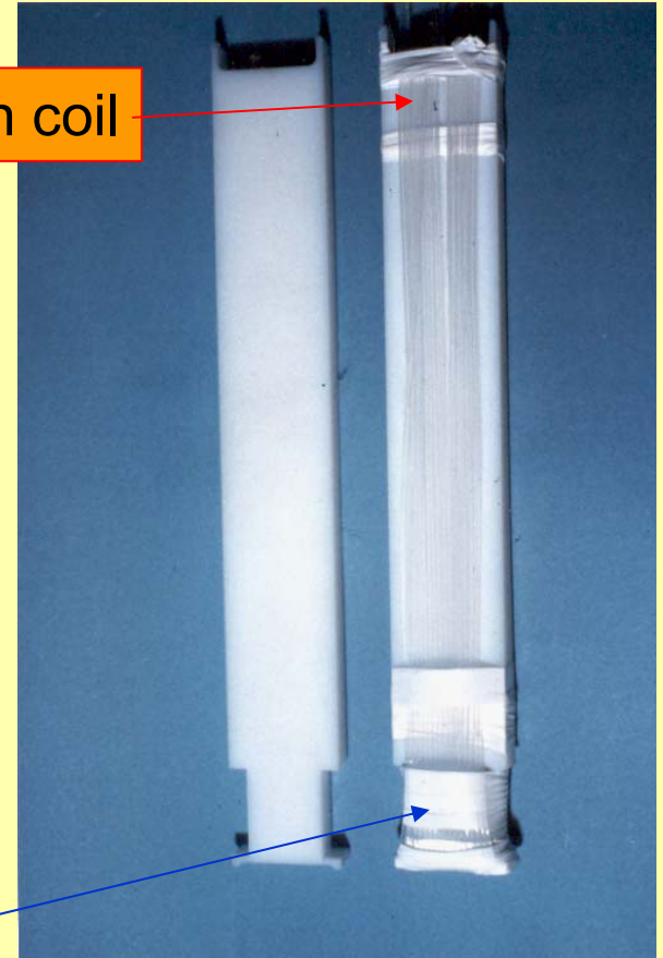
Fig. 2 PTFE shaft (1) with reaction coil (L2) and 'dummy load' coil (L3) wound in two perpendicular planes as detailed in the text. The upper part of the shaft (A) is situated in the chimney of the MWD while the lower part (B) resides within the irradiated zone of the MWD. Two orientations of the shaft within the MWD are possible: a-b ('parallel') and c-d ('perpendicular')
