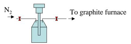
With direct transport and trapping in the atomizer
