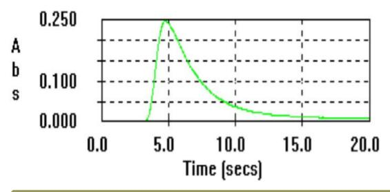
Calibration line: Y=0,0405×[Hg] + 0,0079 Linearity: 10 ng/mL Detection limit: 0,1 ng/mL Repeatability: 4.4% (peak height)
