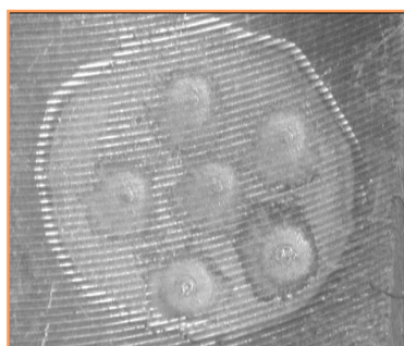
Several laser shots on a single, dried, 10 \mu\text{L} sample droplet
