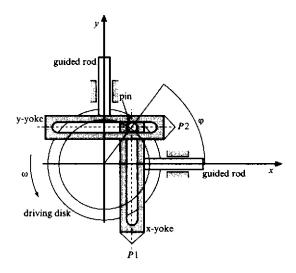
Figure 6.6: Scotch yoke mechanism
