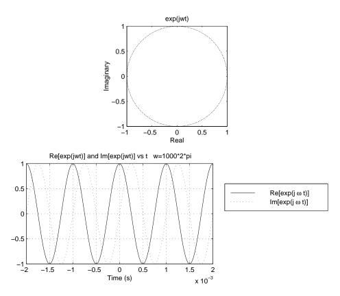
Figure 6.5: The signals  $e^{j\omega t},$  Re  $\left[e^{j\omega t}\right],$  and Im  $\left[e^{j\omega t}\right]$
