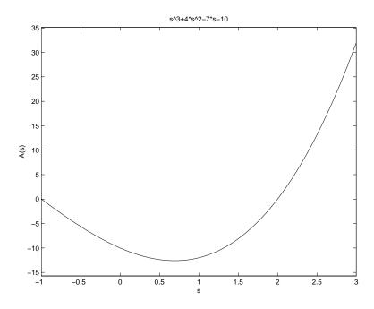
Figure 13.1: Plot of a polynomial function using ezplot
