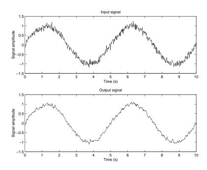
Figure 8.3: 3-point moving average signal filtering
