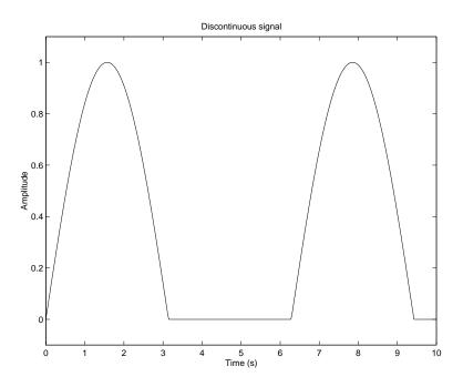
Figure 8.1: Plot of a discontinuous signal
