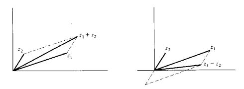
Figure 4.5: Addition and subtraction of complex numbers
