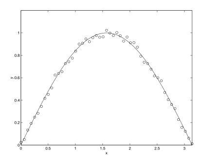
Figure 11.8: Measurements of a sine signal containing Gaussian distributed random errors
