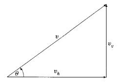
Figure 1.1: Initial velocity (v) divided into horizonal  $(v_h)$  and vertical  $(v_v)$  components.
