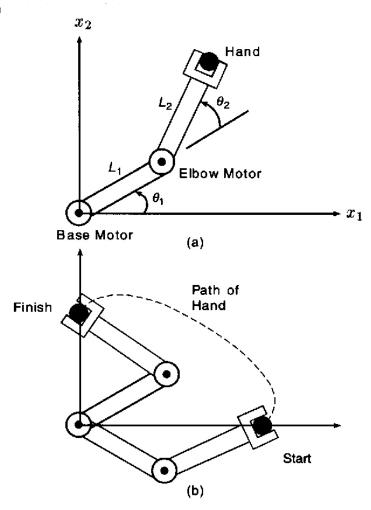
Figure 9.6: Robot arm
