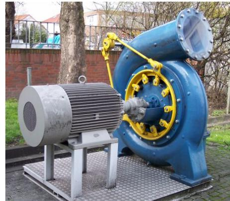
*Exterior view of a Francis turbine attached to a generator (source: Wikimedia Commons CC BY-SA 3.0)*
